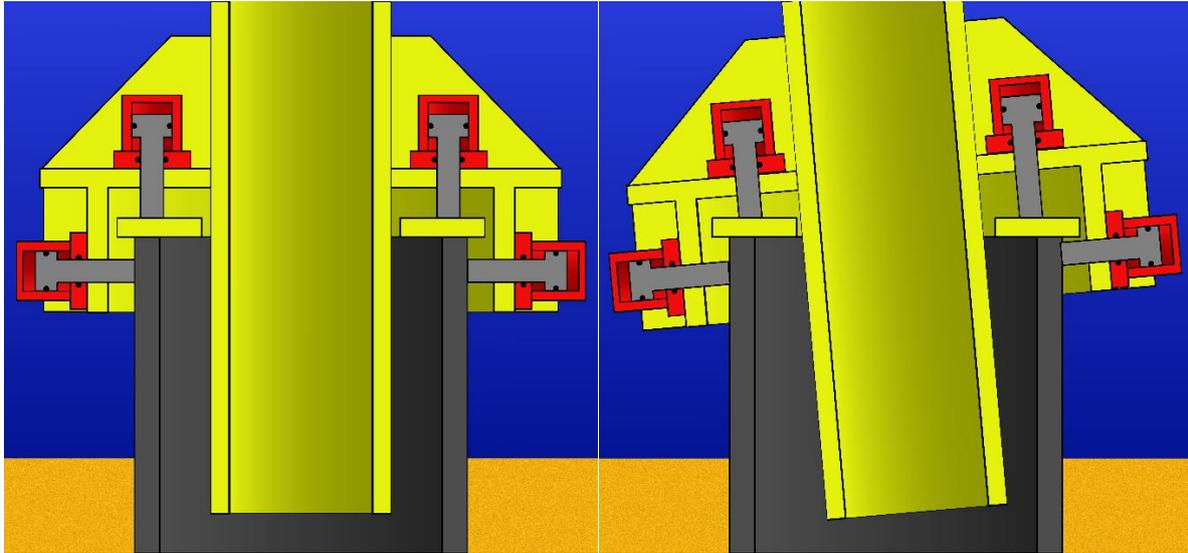
The conventional pile gripper utilised gripping cylinders in a horizontal and vertical configuration at the top of the pile and around the jacket structure; however, this does not address relative motion where the jacket leg protrudes into the pile.
