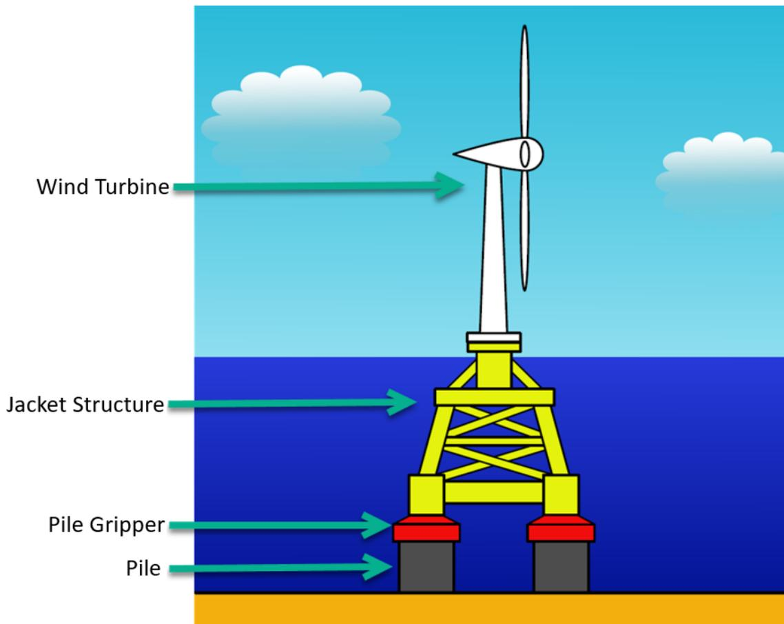
The movement of the jacket leg relative to the pile gripper, referred to as Early Age Cycling, can lead to crack formation within the grout when allowed to take place beyond the specified allowable distance. This crack can significantly reduce the structure's performance and lead to reduced shear capacity of the configuration. Future systems, therefore, require modification to ensure they remain secure for their intended lifespan.
