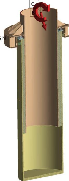
The objective of the analysis was to determine the maximum relative movement between the pile and the jacket leg; this was obtained by probing nodal displacement.
